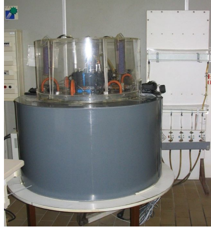
Figure A2-4 : Laboratory equipment for the frost swelling test 0/5mm of the Nancy's Public works regional laboratory
