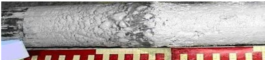
Figure A2-2: Swelling of a chalky soil sample created by the frost
